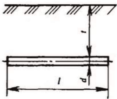
$$\left. \begin{array}{l} R = \frac{\rho}{2\pi l} \ln \frac{l^2}{dt} \text{ — цилиндр} \\ R = \frac{\rho}{2\pi l} \ln \frac{2l^2}{bt} \text{ — полоса} \\ \text{шириной } b \end{array} \right\}$$
